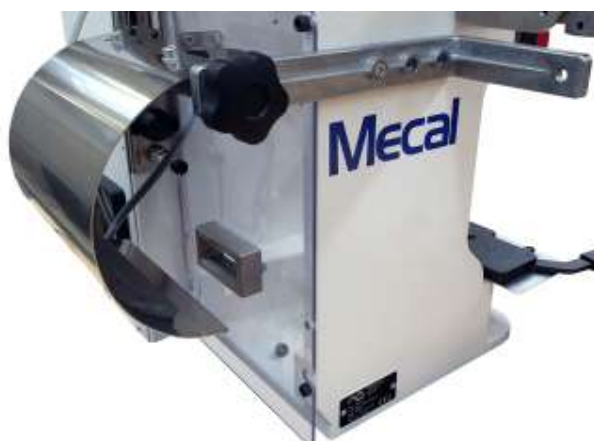
Detail of positioning of the lower conveyor in the rear reel loading condition.
